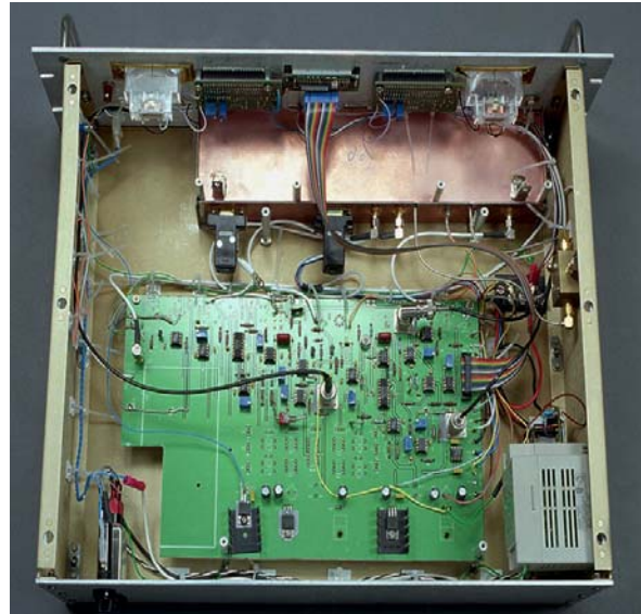
Fig. II-7. RF feedback controller chassis for RIA 350 MHz resonators
